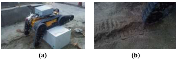
Notes: (a) Climbing over 0.38m obstacle successful; (b) track teeth marks
